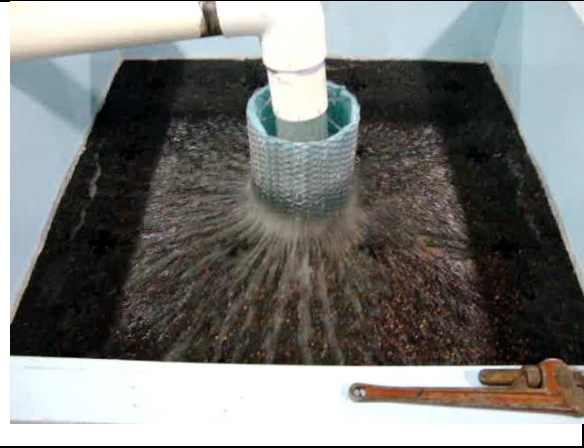
Figure 3. Drain holes open, 25 gpm/tile
