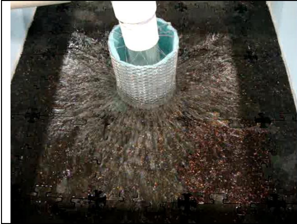
Figure 2. Drain holes open, 2.5 gpm/tile
