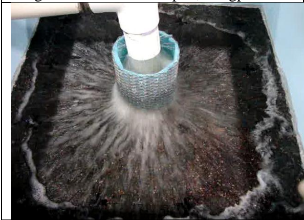
Figure 4. Drain holes open, 37.5 gpm/tile
